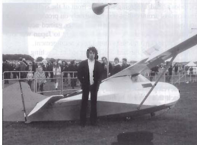
The Hütter at Aston Down before its restoration in 1979, showing the Fin strake, enclosed canopy, airbrakes and wheel. (Can anyone recognise the gentleman standing in front of the glider?)
